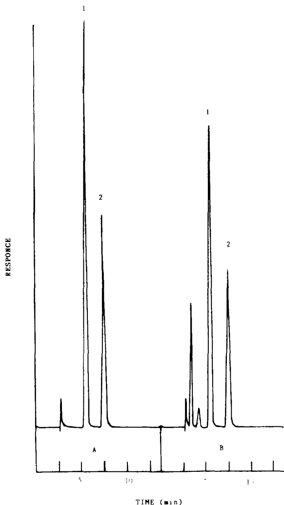
Fig. 4 Liquid chromatograms of (A) furosemide (1) and CSA (2) and (B) a powder sample of furosemide form I exposed to direct sunlight for 240 h in the presence of oxygen.
